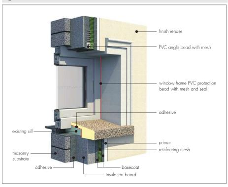
Figure 10 Window opening detail
