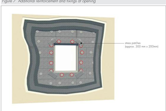
Figure 7 Additional reinforcement and fixings at opening
